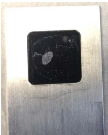
Figure 8: Ketamine and Ethanol Mixture Residue.
