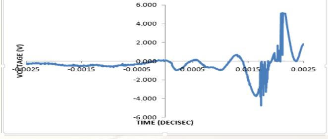
Note: After The Four Boundaries Were Tested, The Output Voltage In Every Single Case showed A Result Peak Voltage of 4.81V From Which 3.40V Is Effective Voltage, Therefore For Simplicity No Boundaries Set Up Was Chosen
