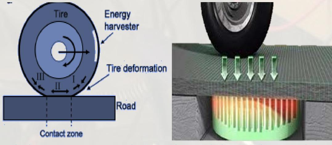
Vehicle Tire Transmits Weight Onto The Road Then To The Piezoelectric Components
